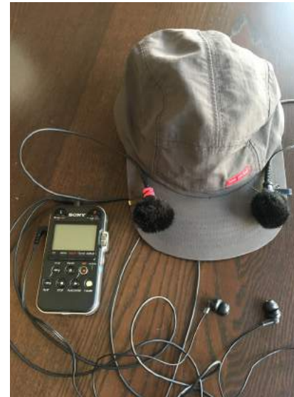
Left: Sound Hat: Sony PCM M-10 Recorder; LOM Instruments Uši Microphones (photo by Ted Gordon).
